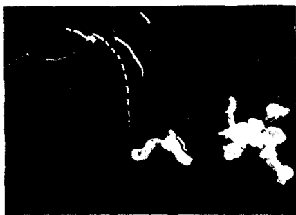
Fig. 3. An electron micrograph of a droplet containing TMV frozen in the usual way but sublimed under poor vacuum. It is an example of the appearance of the networks when pressures of about 11 mm of mercury are used. Note the almost complete aggregation of the networks. Magnification is 35,000. Micrograph prepared by Y. CHEN.
